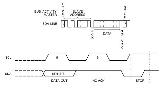
Figure 9. Immediate Address Read Timing
