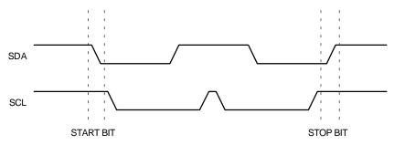
Figure 4. Start/Stop Timing
