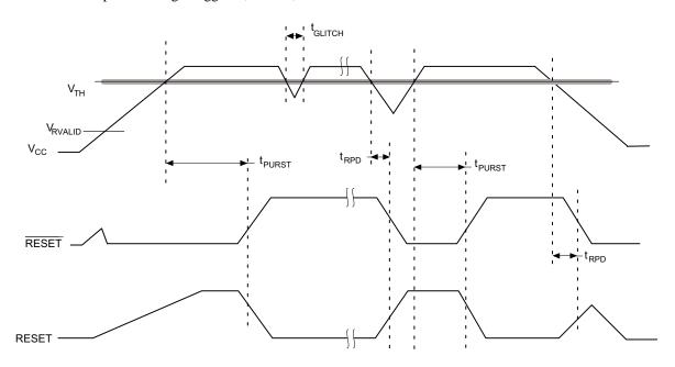
Figure 1. RESET Output Timing
