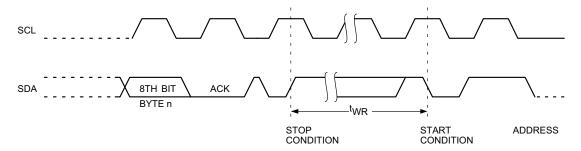
Figure 3. Write Cycle Timing
